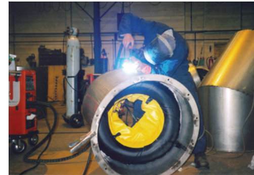
Rapid Purge used to weld a stainless steel elbow.
